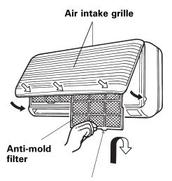
Insert into the groove on the unit.
